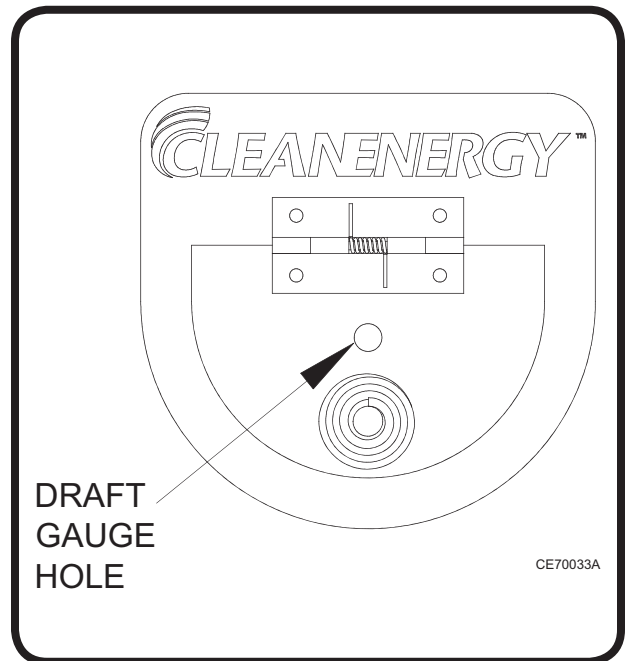
Figure 26: Draft Gauge Hole in the Observation Port
